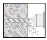
Drilling of hole with an electric drill to the diameter and depth required by the selected reinforcing bar. In case of aborted drill hole: the drill hole shall be filled with mortar.
